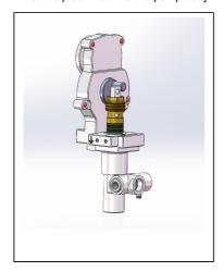
3. Tighten the copper sleeve.
