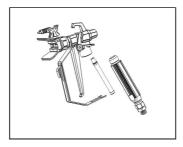
2. Remove spray tip and tip guard and clean with water or flushing fluid and a brush.
