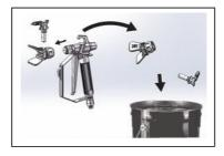
3. Wipe paint off outside of gun using a soft cloth moistened with water or flushing fluid.
