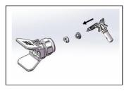
Spray tip must be pushed all the way into the tip guard.
